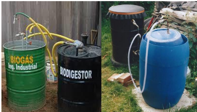
Examples of small, homemade anaerobic digesters.
